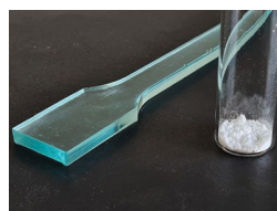
(3) Roizefar epoxy resin BPA content: approx. 30 wt%
