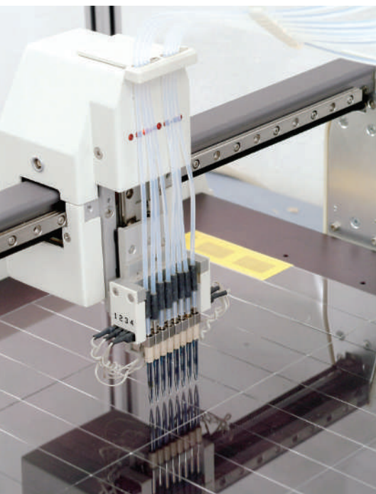
JPT uses a high-throughput, non-contact printing process to assemble its peptide arrays.
