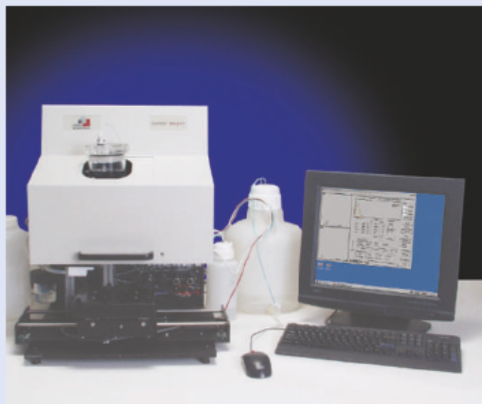
Union Biometrika's BioSorter COPAS can sort clusters of cells.
