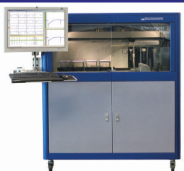
Aviva's SealChip16 for patch-clamping (above) is the heart of its PatchXpress7000 system (left) for assaying ion channels.
