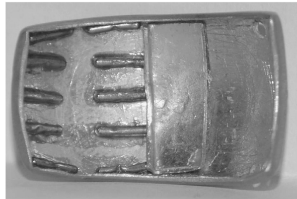
Figure 9 I-125 plaque showing anterior unloaded extension.
