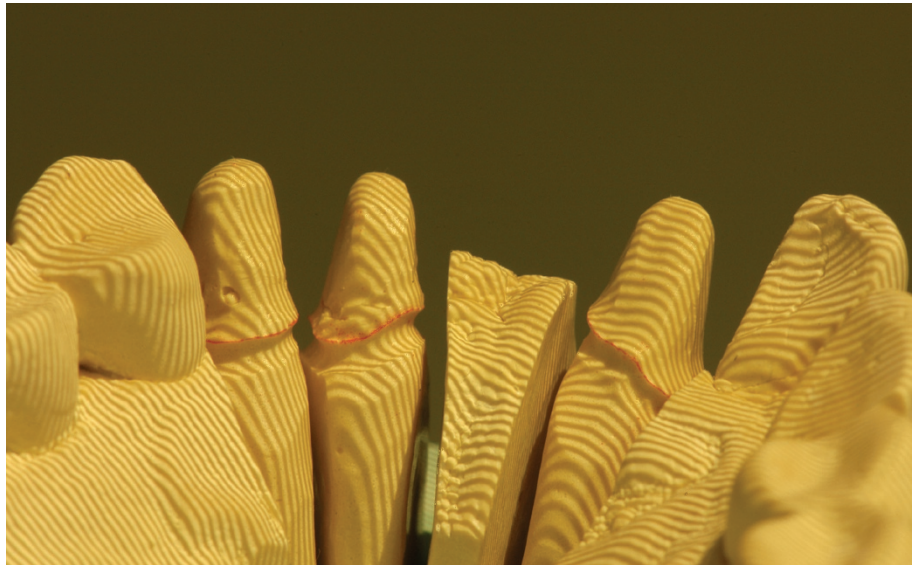
Fig. 1 White light projector pattern during the scanning process by an optical scanner
