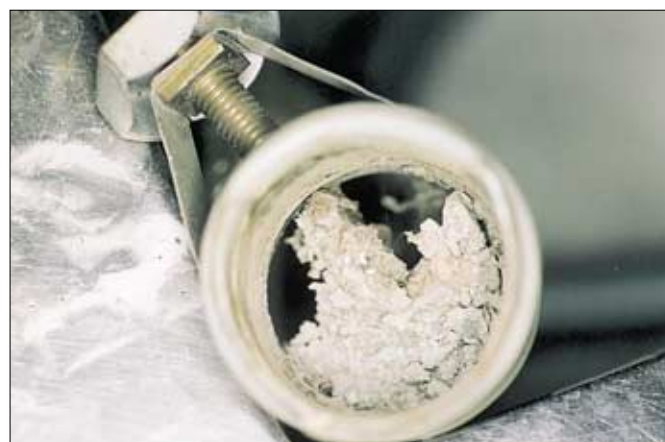
Fig. 5 Photograph of amalgam contamination within corrugated internal tubing of aspirator.
