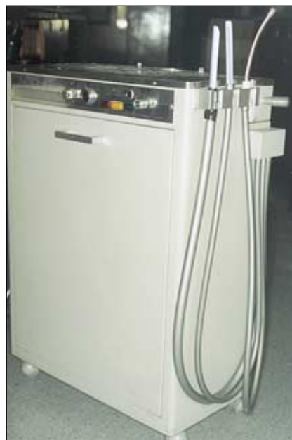
Fig. 1 Photograph of the aspirator under investigation. This particular model was of the self contained and semi-mobile trolley type that is designed to be plumbed-in next to the dental chair. This aspirator expelled its waste air through four holes in the base of the unit and consequently released mercury vapour into the breathing zone.
