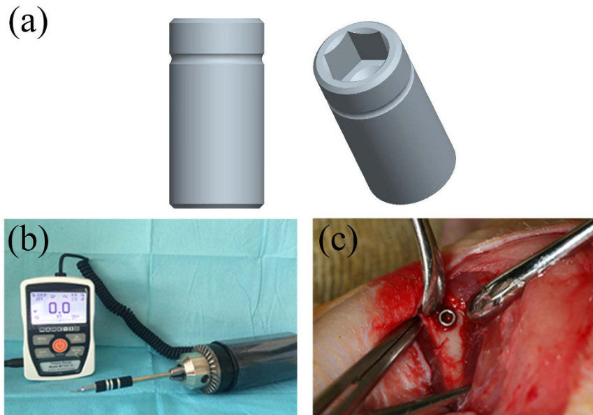
Figure 8. The pattern of the experimental implants, the engaging torque-testing machine and the intraoperative location of implants. (a) The pure titanium cylindrical implants. (b) The torque-testing machine. (c) The implants are placed into the distal metaphysis of bilateral femurs where the notch is at the bone level.
