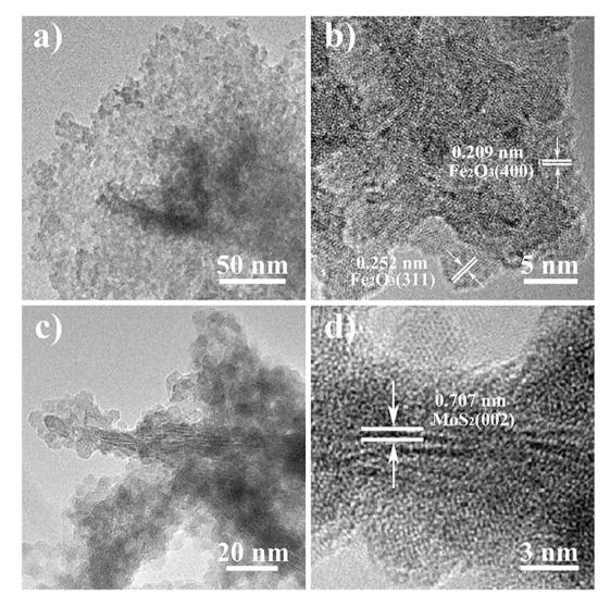
**Figure 2. TEM image of Fe<sub>2</sub>O<sub>3</sub>/MoS<sub>2</sub> composite.** (**a**,**b**) TEM and HRTEM images taken from basal plane, and (**c**,**d**) cross-section TEM and HRTEM image of basal plane.
