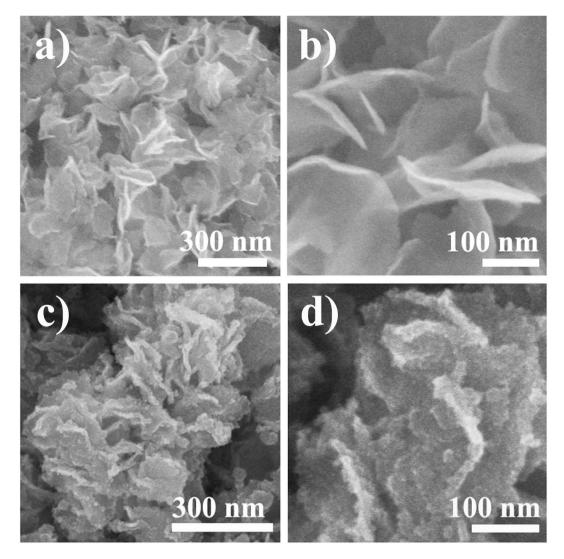
Figure 1. Structrual characterization of  $MoS_2$  nanosheets and  $Fe_2O_3/MoS_2$  composite. (a,b) SEM of  $MoS_2$  nanosheets, and (c,d) SEM of  $Fe_2O_3/MoS_2$  composite.
