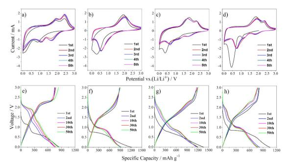
**Figure 5.** CV curves of (**a**) MoS<sub>2</sub> nanosheets, (**b**)  $Fe_2O_3$ , (**c**)  $Fe_2O_3/MoS_2$  composite and (**d**) the physical mixture  $Fe_2O_3 + MoS_2$ , and charging-discharging curves of (**e**) MoS<sub>2</sub> nanosheets, (**f**)  $Fe_2O_3$ , (**g**)  $Fe_2O_3/MoS_2$  composite and (**h**) the physical mixture  $Fe_2O_3 + MoS_2$ .
