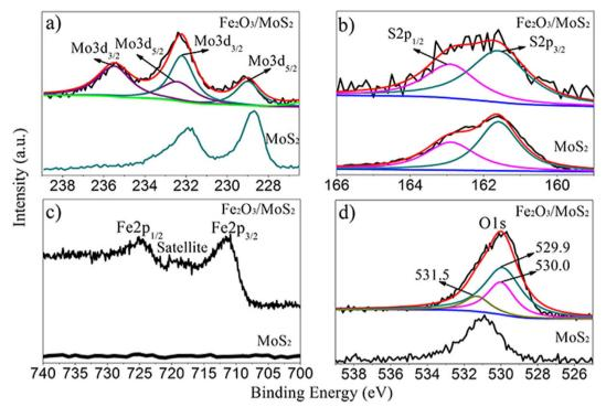
**Figure 4.** XPS spectra of Fe<sub>2</sub>O<sub>3</sub>/MoS<sub>2</sub> composite and MoS<sub>2</sub> nanosheets. (a) Mo 3d XPS spectrum, (b) S 2p XPS spectra, (c) Fe 2P XPS spectrum, and (d) O 1 s XPS spectrum.
