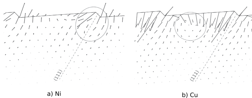
Figure 2. Displacement fields of Ni(1 1 1) and Cu(1 1 1) surfaces are shown. Arrows show the displacements of the atoms from their bulk positions (multiplied by 100 for clarity). Surface atoms are traced by grey lines. Dashed lines mark the (111) planes. The general regions of the displacement vortices are circled. In the case of the Ni(1 1 1) surface (a) some of the terrace atoms are displaced towards the bulk and others away from the bulk. The step corner and terrace edge atoms are displaced the most and the atoms in the middle of the terrace are displaced the least. The vortex is centered on the (111) plane marked with a dashed line. In the case of the Cu(1 1 1) surface (b) all the terrace atoms are displaced towards the bulk, whereas the step corner atom is displaced outwards. The displacements form a vortex underneath the terrace.
