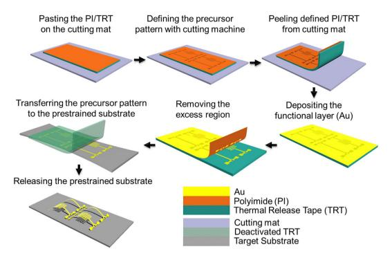
Figure 1. The fabrication process of the "Cut-Transfer-Release" method.
