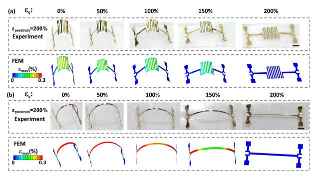
Figure 2. The optical images and FEM strain distribution results of 3D structures during releasing the 200% prestrained substrate. (a) the 3D Au/PI serpentine-like structure (b) the 3D Au/PI ribbon structure (scale bar: 1 mm).
