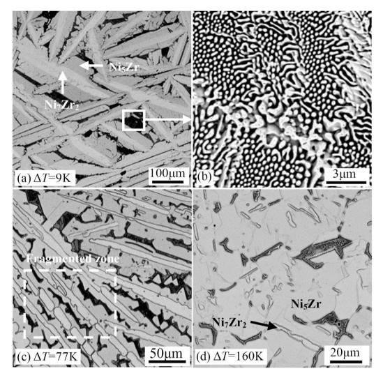
**Figure 3.** Solidified microstructures of undercooled Ni<sub>83.25</sub>Zr<sub>16.75</sub> peritectic alloy at undercooling of (**a**,**b**)  $\Delta T = 9$  K, (**c**)  $\Delta T = 77$  K, and (**d**)  $\Delta T = 160$  K.
