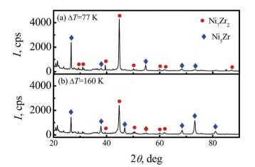
**Figure 4.** XRD patterns of samples solidified at undercoolings of (a)  $\Delta T = 77$  K and (b)  $\Delta T = 160$  K to reveal the volume change of the two phases.
