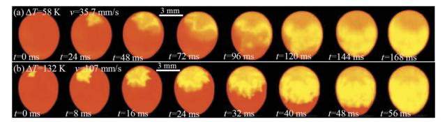
Figure 1. High-speed camera images of recalescence front of undercooled Ni<sub>83.25</sub>Zr<sub>16.75</sub> peritectic samples at different undercoolings. The red part is the undercooled liquid, and the yellow part is the recalescing solid. The time interval between two adjacent images is 24 ms and 8 ms, respectively. (a)  $\Delta T = 58$  K; (b)  $\Delta T = 132$  K.
