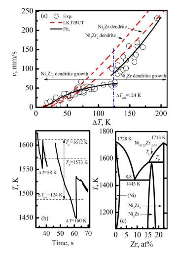
Figure 2. (a) Dendritic growth velocity versus undercooling. (b) Temperature-time recalescence characteristics at different undercoolings. (c) The left part of Ni-Zr binary phase diagram<sup>24</sup>.
