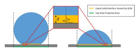
Figure 2. Schematic of the comparison between top view projected area observed by microscope and liquid/solid interface sensed by QCM on different surfaces. The inset is the resonant shear acoustic wave decaying within propagation thickness at liquid/solid interface.
