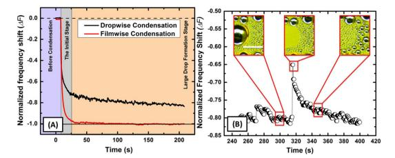
**Figure 5.** (A) Resonant frequency shift signal of dropwise and filmwise condensation on flat surfaces: (i) before condensation, (ii) the initial stage of condensation, and (iii) the large drop formation stage; (B) The detail QCM frequency signals and correlated microscopic images about interfacial area fluctuation (The scale bar of the inset images is 1 mm).
