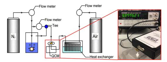
Figure 4. Schematic of the QCM based measurement system.
