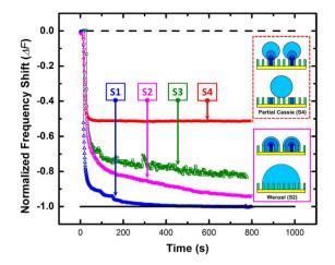
**Figure 8.** Normalized frequency shift signals of condensations on different surfaces (*SP* = 1.72). The insets are the droplet growth mechanisms of Wenzel and partial Cassie DWC.
