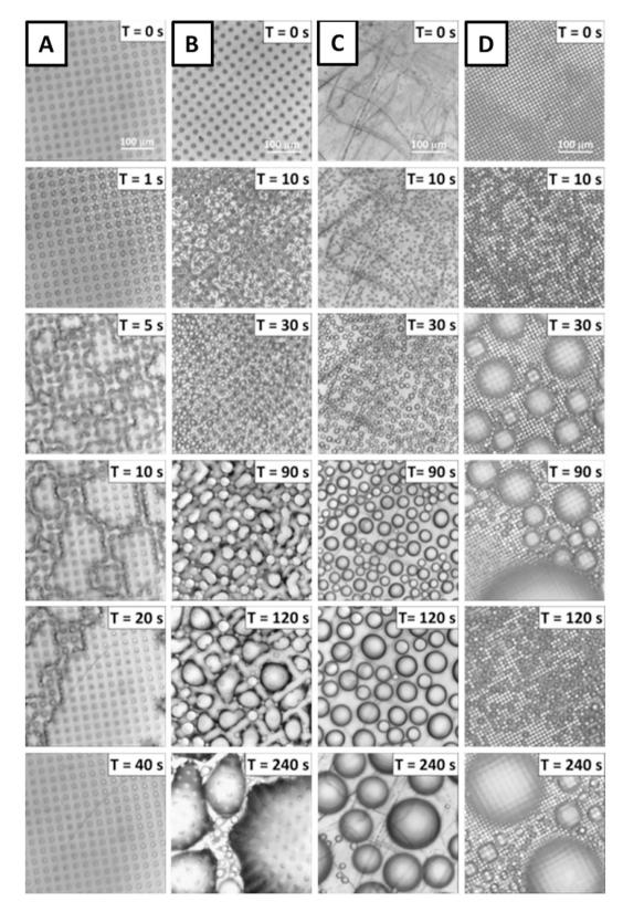
**Figure 7.** Time advancing optical microscopic images of condensations on different surfaces at SP = 1.72: (A) filmwise condensation on a hydrophilic micropillar surface (S1), (B) Wenzel dropwise condensation on a hydrophobic micropillar surface (S2), (C) dropwise condensation on a flat hydrophobic surface (S3), and (D) partial Cassie dropwise condensation on a hydrophobic micropillar surface (S4).
