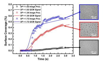
Figure 6. Comparison of drop-surface interface obtained from direction observation (optical microscope) and QCM measurement for different saturation points (SP = 1.02, 1.37, and 1.72).
