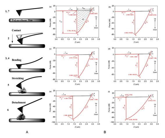
**Figure 7.** The diagram of nanomechanical properties of WPU by AFM. (A) Sketch of the seven stages reflecting the variation of WPU films during the force spectroscopy experiment. (B) (a–f) Experimental forcedistance curves for a trace and retrace for samples I-WPU, IW-WPU, S-WPU, W-WPU1, W-WPU2, W-WPU3, respectively; the stages labeled on the curves corresponds to the sketch of seven stages. The meanings of  $F_{\text{max}}$ ,  $d_{\text{max}}$  and W are also identified in (a).
