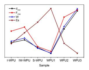
Figure 8. Trends of the maximum distance of deformation  $(d_{max})$ , maximum adhesive force  $(F_{max})$ , adhesion energy (W) and Young's modulus  $(E_s)$  of the WPU samples.
