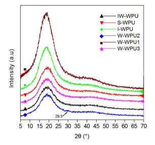
Figure 4. X-ray diffractograms of the WPU films.
