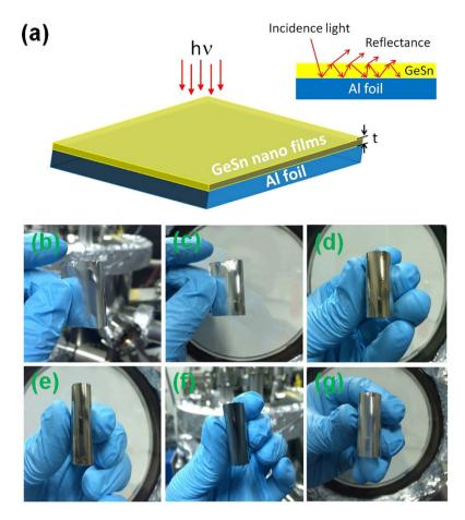
**Figure 1.** (a) Schematic of the GeSn nano films with thickness of *t* coating on Al foils. (**b**–**g**) Widely color spectra of the nanometer GeSn coating on Al foils, t = 0, 20, 40, 60, 100 and 180 nm (Photos are taken under illumination from conventional fluorescent ceiling lights).
