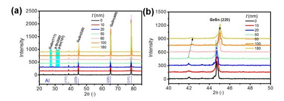
**Figure 3.** (a) XRD patterns of GeSn nanometer coating on Al foil. (b) Enlarged XRD patterns with  $2\theta$  ranging from  $40^{\circ}$  to  $50^{\circ}$ .
