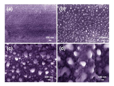
**Figure 4.** High resolution SEM images of GeSn thin film coating on Al foils (**a**) t = 20 nm (**b**) t = 50 nm (**c**) t = 100 nm (**d**) t = 180 nm.
