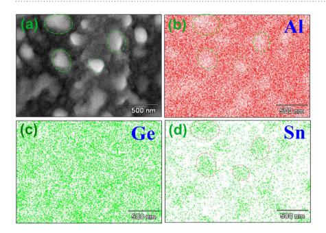
**Figure 5.** EDS of GeSn films with a thickness of 180 nm grown on Al foil (**a**) SEM image of GeSn with a thickness 180 nm grown on Al foil. (**b**) Al element mapping. (**c**) Ge element mapping. (**d**) Sn element mapping.
