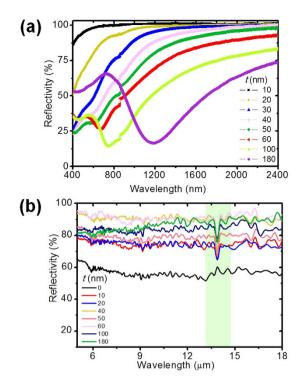
**Figure 6.** (a) Refection spectra (from 400 to 2400 nm in wavelength) of Al foil coated with 10, 20, 30, 40, 50, 60, 100 and 180 nm of GeSn thin films. (b) Refection spectra (from 5 to  $18 \,\mu$ m in wavelength) of Al foil coated with various thickness of GeSn thin films.
