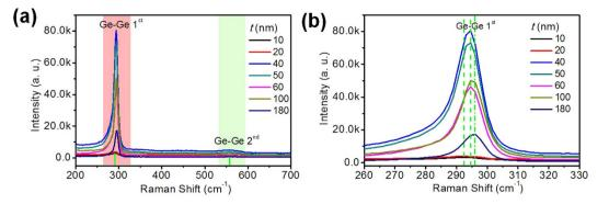
**Figure 2.** (a) Micro-Raman spectroscopy measurement for the nanometer GeSn thin films coating on Al foil with different *t*. (b) Enlarged Ge-Ge peak shift as function of GeSn thickness.
