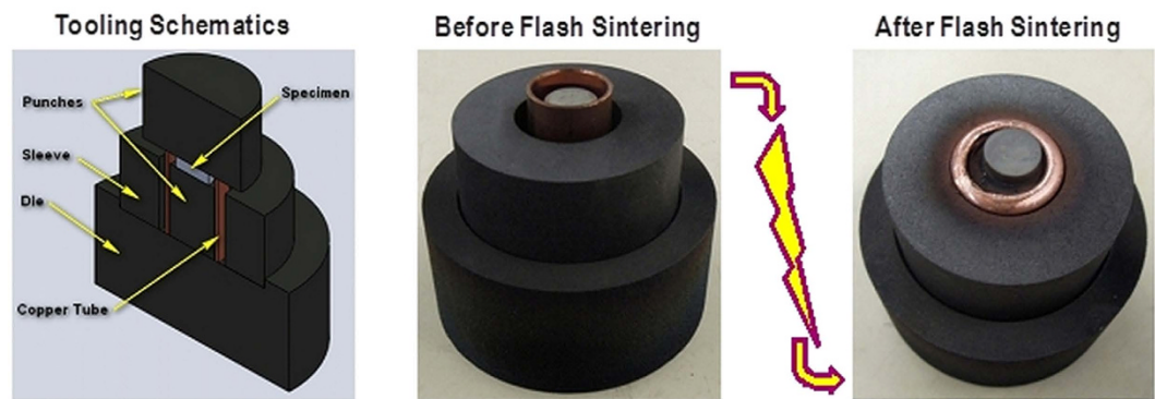
Figure 1. Shown above is the FHP die system. These dies allow the specimen to be isolated from electrical current while being heated through radiation heating. At critical temperature, the copper tube collapses and the specimen is exposed to the current of the SPS device.
