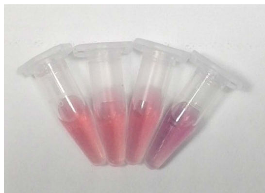
Figure 3. Photograph of color changes caused by adding HBeAg to aptamer-linked AuNPs. From left to right: aptamer-linked AuNPs + 0.09 M NaCl; aptamer-linked AuNPs + 50 nM parenzyme + 0.09 M NaCl; aptamer-linked AuNPs + 50 nM HBeAg + 0.09 M NaCl; aptamer-linked AuNPs + 50 nM HBeAg + 0.09 M NaCl.
