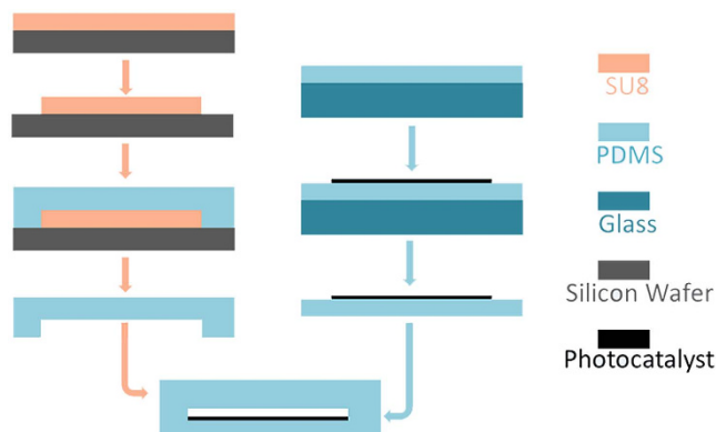
Figure 9. Procedure for the fabrication of the microreactor chip.
