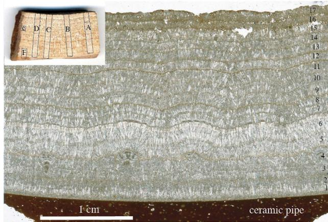
**Figure 2. Investigated sample.** Thin section of sample P2, showing a regular alternation of thick microsparite and thin micrite layers. Notice the slight curvature of the sample, which followed the large diameter of the siphon pipe. Layers are numbered corresponding to peaks in stable isotopes (Fig. 3). Inset: the original sample with micromill traces of Fig. 3.
