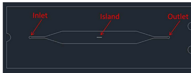
Figure 5. Shows a top view of the channel design in the chip, with an elliptical island in the middle.
