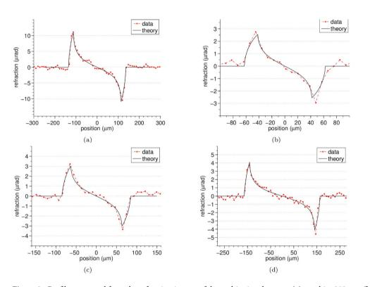
**Figure 3.** Profiles extracted from the refraction images of the multi-wire phantom: (a) sapphire 250  $\mu$ m, (b) Nylon 100  $\mu$ m, (c) PEEK 150  $\mu$ m and (d) Nylon 300  $\mu$ m diameter.
