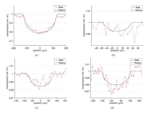
**Figure 4.** Profiles extracted from the attenuation images of the multi-wire phantom: (a) sapphire 250  $\mu$ m, (b) Nylon 100  $\mu$ m, (c) PEEK 150  $\mu$ m and (d) Nylon 300  $\mu$ m diameter.
