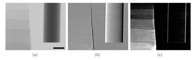
Figure 5. (a) attenuation, (b) refraction and (c) scattering contrast images of the acrylic rod and paper step wedge sample. Scale bar is 2 mm.
