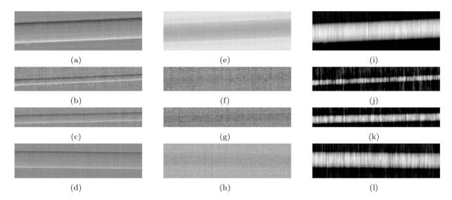
**Figure 2.** Images of the multi-wire phantom: (**a**–**d**) refraction, (**e**–**h**) attenuation and (**i**–**l**) phase. From top to bottom: sapphire  $250 \,\mu\text{m}$ , Nylon  $100 \,\mu\text{m}$ , PEEK  $150 \,\mu\text{m}$  and Nylon  $300 \,\mu\text{m}$  diameter. The vertical stripes that can be seen in panels (**i**–**l**) run parallel to the direction of integration and are a result of the presence of noise in the integrand images (**a**–**d**).
