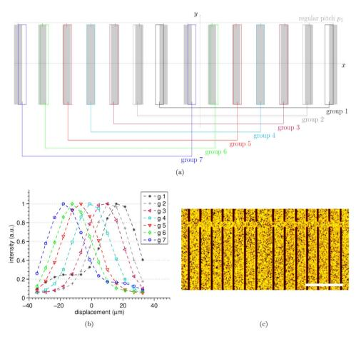
Figure 7. 7-way asymmetric aperture pattern. (a) schematic of the design, (b) experimental illumination functions and (c) optical microscope image, scale bar is  $250 \, \mu \text{m}$ . At the mask position corresponding to  $0 \, \mu \text{m}$  displacement, seven complementary illumination conditions  $\pm 35\%$ ,  $\pm 60\%$ ,  $\pm 80\%$  and 100% are obtained.
