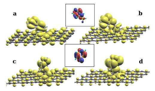
**Figure 4.** Panels (**a**,**b**) plot the MIDGAP-l and MIDGAP-h states, respectively, formed by hybridizing the mid gap state of graphene with the LUMO of core-excited 4-picoline radical, and showing mostly bonding and antibonding amplitude contours, respectively. Panels (**c**,**d**) show the same states for a core-excited pyridine radical. Gas phase LUMO for 4-picoline and pyridine are plotted in the insets.
