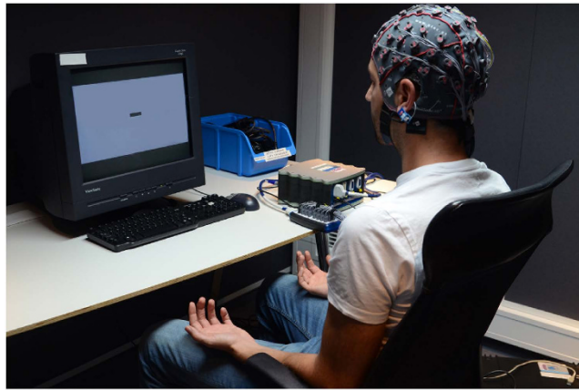
Figure 5. Experimental setup during EEG acquisition and BMI-control: A 64-channel EEG system was used for recording brain activity. During motor imagery and BMI control, the instructions and the visual stimuli, including the BMI feedback as shown in the picture, were presented on a computer screen. Participants sat comfortably in front of the screen, keeping their hands on their thighs with the palms up.
