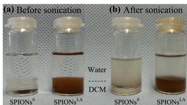
Figure 3. Photos of SPIONs 0 and SPIONs LA in water/DCM: (a) just after adding DCM and water, (b) 2 min after sonication.
