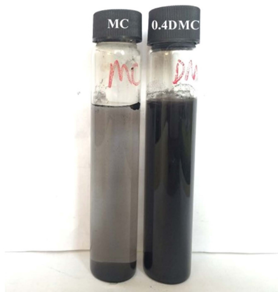
Figure 5. Photographs of the dispersions of 0.4DMC-550 and MC-550 in water, after sonication for 5 min and storage for 10 min under ambient conditions.
