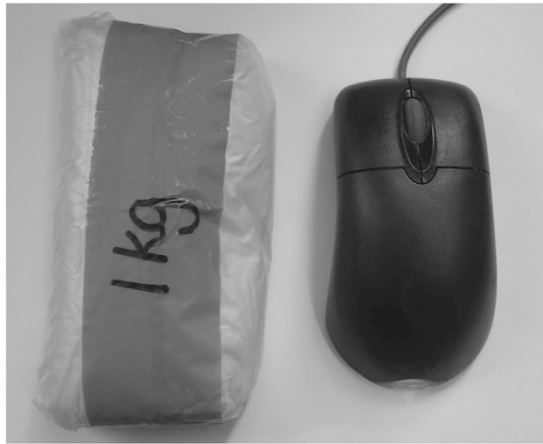
Figure 1. Innovative MR-compatible high density material barium sulfate. Barium sulfate ( \text{BaSO}_4 ) of mass 1 kg placed within a sealed freezer bag (shown next to a computer mouse for context).
