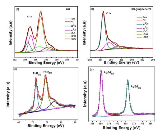
Figure 3. XPS spectra of the (a) GO, (b) 3D-graphene/Pt, (c) Pt  $4f_{7/2}$  and Pt  $4f_{5/2}$  peaks of 3D-graphene/Pt and (d) Ag  $3d_{5/2}$  and  $3d_{3/2}$  peaks in 3D-graphene/Ag nanocomposites.
