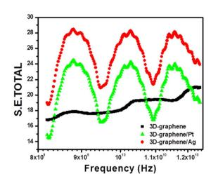
Figure 7. EMI shielding effectiveness (dB) of 3D-graphene, 3D-graphene/Pt, and 3D-graphene/Ag nanocomposites.
