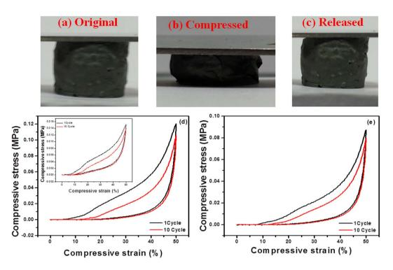
**Figure 6.** Compressibility of 3D-graphene, 3D-graphene/Pt, and 3D-graphene/Ag naocomposites. (a–c) Digital images of a typical compression process of 3D-graphene/noble metal nanocomposites. Compressive stress-strain curves of 10 cycles (loading and unloading) of (d) 3D-graphene/Pt and (e) 3D-graphene/Ag nanocomposites (Inset: Compressive stress-strain curve of 3D-graphene).
