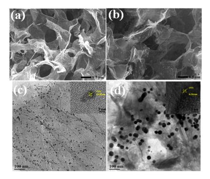
**Figure 4.** FEG-SEM images of (a) 3D-graphene/Pt and (b) 3D-graphene/Ag nanocomposites; TEM and HRTEM images of (c) 3D-graphene/Pt and (d) 3D-graphene/Ag nanocomposites.
