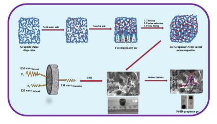
Figure 1. Schematic representation of 3D-graphene/noble metal nanocomposites by the freeze-casting method, and its application in EMI shielding and electrocatalytic oxidation of methanol.
