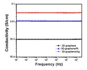
Figure 5. Frequency-dependent real part of AC conductivity of 3D-graphene, 3D-graphene/Pt, and 3D-graphene/Ag nanocomposites.
