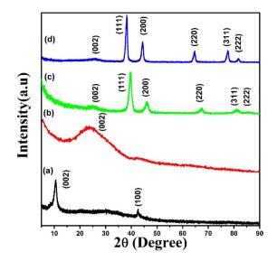
Figure 2. XRD patterns of (a) GO, (b) bare 3D-graphene, (c) 3D-graphene/Pt and (d) 3D- graphene/Ag nanocomposites.
