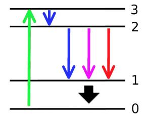
**Figure 2.** Sketch of a 4-level laser rate system. Sinuous lines represent electronic procedures due to 2-photon pumping, the excitation (green). Level 2 to 1: spontaneous emission (blue), stimulated emission (bright pink) and phonons (red).
