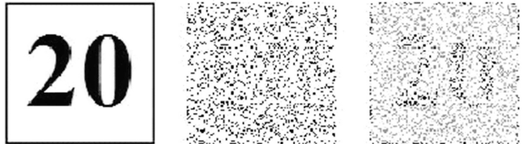
Figure 2. (a) Original image, (b) pulse and high noisy image (c) output image.
