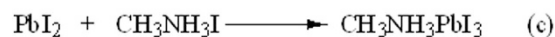
Figure 4. The mechanism to form the perovskite from PbO and CH 3 NH 3 I.
