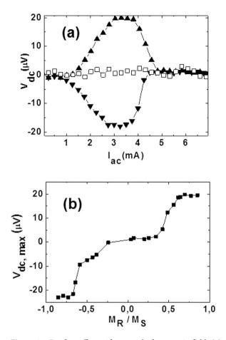
**Figure 2.** Ratchet effect without applied magnetic field: (a) dc voltages (Y-axis) as a function of the applied ac currents (X-axis) for  $M = M_Z$  (upward triangles),  $M = -M_Z$  (downward triangles) and M = 0 (hollow squares);  $M_Z/M_S = 0.65$  ( $M_s$  being the magnetization at saturation); (b) Maximum dc voltage (Y-axis) as a function of the normalized remanent magnetization (X-axis) for T = 8.45 K. ac current frequency is 10 kHz.
