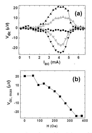
Figure 3. Ratchet as a function of the applied magnetic field. (a) dc voltages (Y-axis) as a function of the applied ac currents (X-axis) at T = 8.45 K and ac current frequency 10 kHz, for applied magnetic fields: 54 Oe (upward triangles), 126 Oe (upward hollow triangles), 240 Oe (squares), 306 Oe (downward hollow triangles) and 378 Oe (downward triangles). (b) maximum output dc voltages (Y-axis) vs. applied magnetic fields (X-axis).
