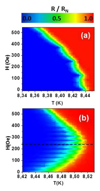
**Figure 4.** Normalized resistance (see color bar) as a function of T (X-axis) and H (Y-axis),  $R_N$  being the resistance taken in the normal state (10 K) and measured with 5  $\mu$ A for: (a) Reference sample: Nb film on top of array of Cu nanodots and (b) Nanodevice: Nb film on top of array of Co/Pd triangles. The dashed line shows the compensation field position.
