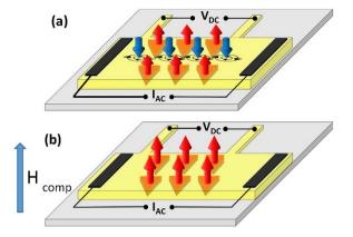
**Figure 1. Sketch of the nanodevice.** Co/Pd multilayer triangular–shaped nanomagnets (orange). Nb thin film (yellow), Si substrate (green) (sketch not to scale). Out of plane magnetization (red arrows). Superconducting vortices (blue arrows). H is the applied magnetic field. (a) H = 0, (b)  $H \neq 0$ , in the case  $H = H_{comp}$ .  $H_{comp}$  being the magnetic field needed to annihilate the interstitial vortices.
