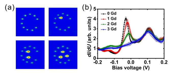
**Figure 4.** The step-by-step evolution of spectroscopy. (a) STM images of the 8.5-nm open Fe corral with 0, 1, 2 and 3 Gd adatoms trapped inside. The image sizes are  $15 \times 15 \, \text{nm}^2$ . (b) The evolution of the STS at the center of the corral during the trapping of Gd adatoms.
