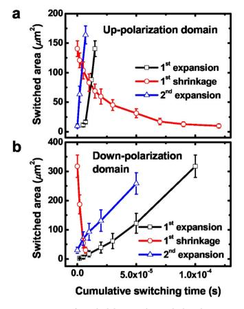
**Figure 5.** Areas of switched domains during the breathing DW motion. a,b The areas of switched domains plotted as a function of cumulative switching time for up- (bright regions) (a) and down-polarization (dark regions) (b) obtained from the PFM images in Fig. 4a,b. The 2nd expansion after the 1st shrinkage of domains does not include the initial nucleation process while the 1st expansion of domains includes the nucleation process.
