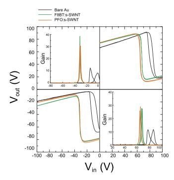
**Figure 8.** Voltage transfer characteristics of ambipolar complementary inverters based on PTVPhI-Eh OFETs [*W*/*L* ratios for *p*- and *n*-channel, *W*/*L* = 1 mm/20 $\mu$ m]: bare Au S/D electrode (black); and, with F8BT:s-SWNT (green) and PFO:s-SWNT interlayer (yellow).
