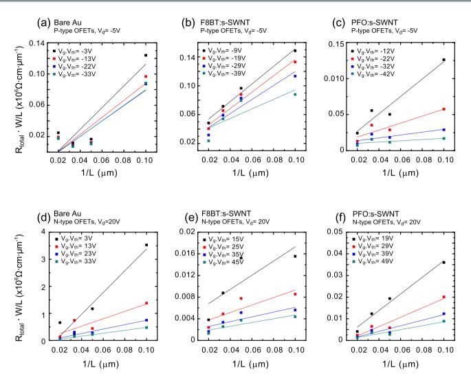
**Figure 6.** Modified transfer-line method plots for *p*- and *n*-channel PTVPhI-Eh OFETs with pristine gold electrodes (**a**, **d**), with F8BT:s-SWNT contacts (**b**, **e**), and with PFO:s-SWNT contacts (**c**, **f**). The slopes of the linear fit denote the  $R_c$ .
