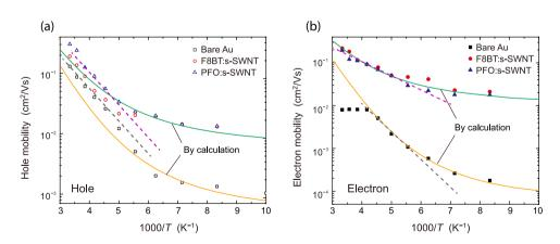
**Figure 7.** Temperature dependence of hole (**a**) and electron (**b**) mobilities and their calculation for OFETs with and without interlayers. Symbols represent experimental results, dashed lines at high temperatures are least-square fittings for extracting activation energy, and solid lines denote calculated data based on a previously reported mobility model.
