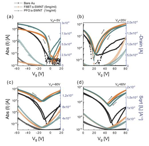
**Figure 2.** *P*-channel and *n*-channel transfer characteristics in linear (**a**,**b**) and saturation (**c**,**d**) regimes of ambipolar PTVPhI-Eh OFETs with s-SWNTs wrapped by F8BT or PFO as a charge-injection interlayer ( $L = 20 \ \mu m$ , W/L = 50,  $C_i = 6.2 \ nFCm^{-2}$ ).
