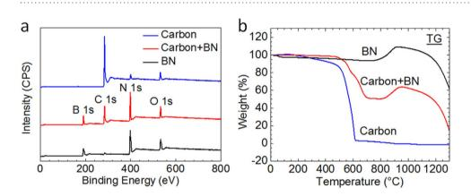
Figure 3. XPS and TG measurements of aerogels. (a) XPS spectra of a carbon aerogel template, a BN/ carbon aerogel and a BN aerogel. (b) The TG analysis for aerogels in  $O_2/N_2$  (1:4) from 0 to 1300 °C.
