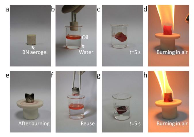
**Figure 8.** Photographs on oil absorption properties of a BN aerogel. (a-d) Absorption and burning process of cyclohexane (stained with Sudan Red II and floating on water) by the BN aerogel within 5 s. (e-h) BN aerogel after burning in air reused for absorption of cyclohexane.
