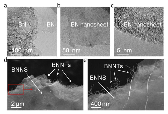
**Figure 6. TEM and SEM images of BN aerogels. (a)** TEM image of a BN aerogel with nanotubes and nanosheets. (b) TEM image of the BN nanosheet. (c) HRTEM of the edge of the BN nanosheet. (d) SEM image of a BN aerogel at lower magnification. (e) SEM image of the BN aerogel at Higher magnification.
