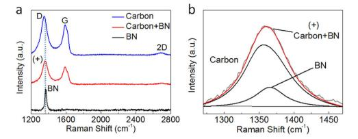
**Figure 2. Raman spectra. (a)** Raman spectra of a carbon areogel template, a BN/carbon aerogel and a BN aerogel. (b) The (+) peak of the BN/carbon aerogel in panel **a** is attributed to two parts—the D peak of carbon and the  $E_{2g}$  vibration peak of BN as fitted by Gaussian curves.
