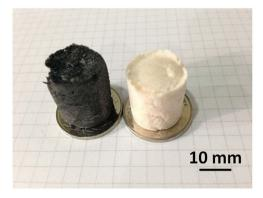
**Figure 1. Photograph.** Carbon aerogel template (left) and BN aerogel (right). The aerogels show significant color change from black to white, which indicates an obvious change in their chemical composition. The BN aerogel maintains the cylindrical shape of the carbon aerogel template.
