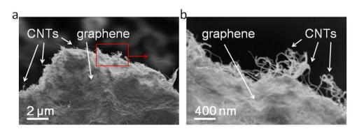
Figure 5. SEM images of a graphene/CNT aerogel. (a) Lower magnification. (b) Higher magnification.
