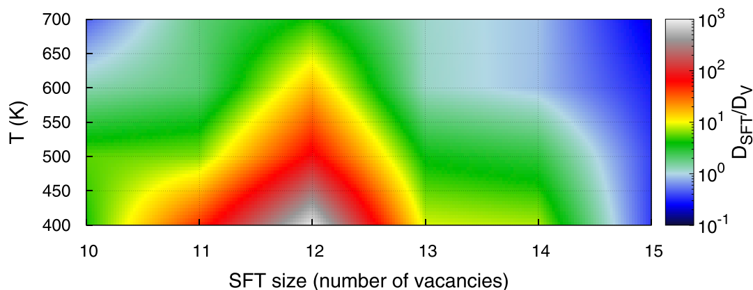
Figure 2 | Map of the diffusion coefficient of a SFT ( D_{SFT} ) relative to the mono-vacancy diffusion coefficient ( D_V ) as a function of its size and temperature, extracted from MD simulations. Temperatures range from 400 to 700 K.
