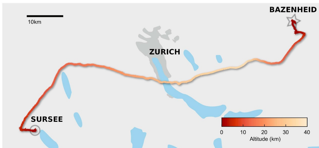
Figure 3 | Flight path of the helium balloon hosting the device under test. The balloon reached a maximum altitude of 35.5 km before bursting. Software used: Gnuplot. Map data: Natural Earth.
