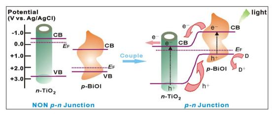
Figure 5 | Schematic diagrams for the energy bands of p-type BiOI and n-type TiO<sub>2</sub> before and after coupling, as well as the specific charge transfer process at the formed p-n junction under visible-light irradiation.
