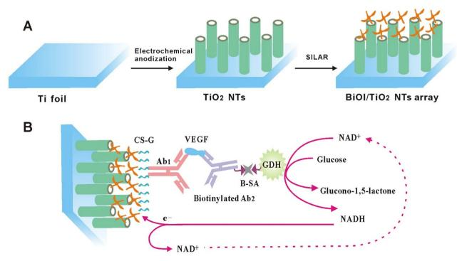
Figure 1 | (A) Schematic Illustration for fabricating crossed BiOI NFs/TiO<sub>2</sub> NTs arrayed structure. (B) Schematic diagram of the immunoanalysis principle using the novel BiOI/TiO<sub>2</sub> NTs arrayed p-n junction photoelectrode.
