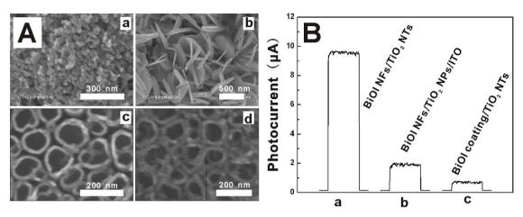
Figure 3 | (A) SEM images of the as-prepared (a) TiO<sub>2</sub> NPs film, (b) BiOI NFs/TiO<sub>2</sub> NPs/ITO, (c) TiO<sub>2</sub> NTs, (d) BiOI film/TiO<sub>2</sub> NTs. (B) The photocurrent responses of the (a) BiOI NFs/TiO<sub>2</sub> NTs, (b) BiOI NFs/TiO<sub>2</sub> NPs/ITO, (c) BiOI coating/TiO<sub>2</sub> NTs. All the tests were performed in 0.10 M PBS containing 0.10 M ascorbic acid with 0 V working potential and 470 nm excitation light.
