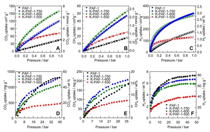
**Figure 2** (A) CO<sub>2</sub> uptake of PAF-1 and KOH-activated samples at 273 K and 1 bar; (B) CH<sub>4</sub> uptake of PAF-1 and KOH-activated samples at 273 K and 1 bar; (C) H<sub>2</sub> uptake of PAF-1 and KOH-activated samples at 77 K and 1 bar; (D) High-pressure CO<sub>2</sub> uptake of KOH-activated samples at 298 K; (E) High Pressure CH<sub>4</sub> uptake of KOH-activated samples at 298 K; (F) High-pressure H<sub>2</sub> uptake of KOH-activated samples at 77 K.
