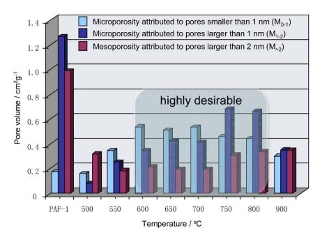
Figure 5 | Pore volume analysis of PAF-1 and KOH activated PAF-1.
