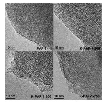
Figure 4 | TEM images of (A) PAF-1 and (B-D) samples activated with KOH at 500°C, 600°C and 750°C, respectively.
