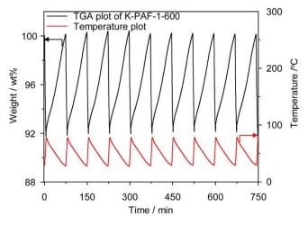
Figure 3 | CO<sub>2</sub> cyclic adsorption (28°C) and desorption (80°C) of K-PAF-1-600. The black curve shows the weight and the red curve is the temperature.
