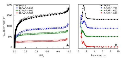
Figure 1 | (A) N<sub>2</sub> sorption isotherms (solid symbols, adsorption; open symbols, desorption) PAF-1 and KOH-activated carbonized PAF-1 derivatives at 77 K; (B) pore size distributions of PAF-1 and KOH-activated carbonized PAF-1 derivatives. The pore size distributions were calculated by the quench solid density functional theory (QSDFT) model.
