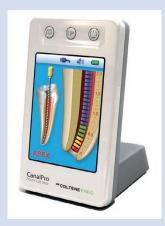
displays a virtual apex function on the LCD colour screen for visual confirmation, but also provides audio feedback for the dentist.
