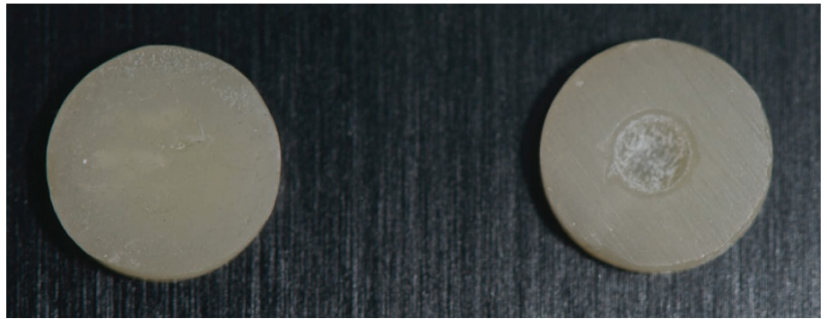
Fig. 1 Composite resin samples without (left) and with (right) porosity
