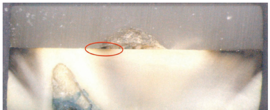
Fig. 5 Example of dentine – composite resin interface of sample restored with composite presenting a porosity subjected to an ambient-pressure environment (Group A2)
