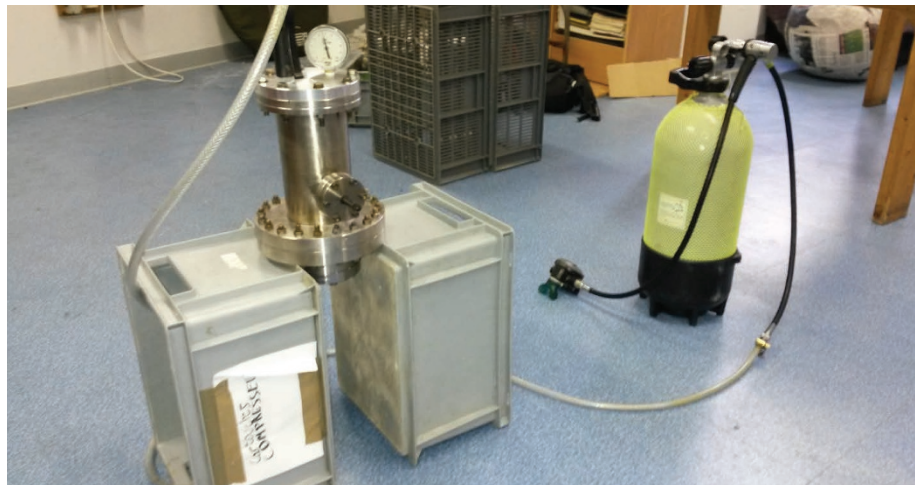
Fig. 2 Hyperbaric simulation apparatus
