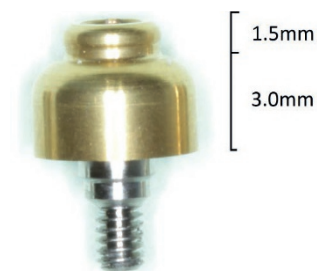
Fig. 22 Straumann Locator Abutment (3 mm Height Wide Neck Locator Abutment) - showing the variable height of the Locator (3 mm height) dictated by the height of the surrounding soft tissue cuff and the standard 1.5 mm working portion that engages into the Locator Male Components
