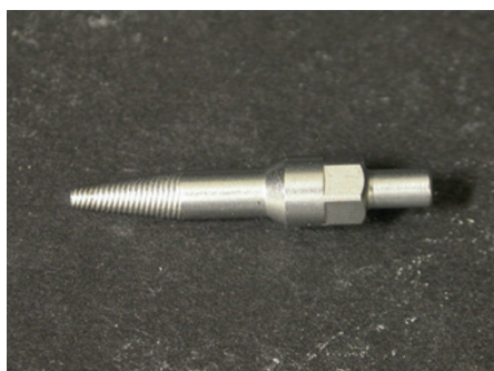
Fig. 1 Reverse screw implant retrieval tool
