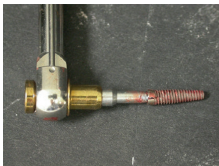
Fig. 2 Retrieval tool with fractured implant attached
