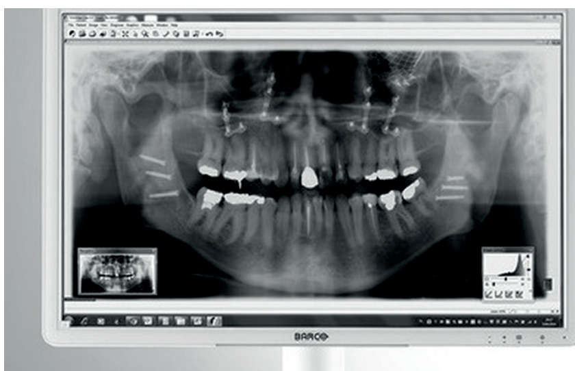
Fig. 4 Dedicated medical grade monitors for dental applications have a stabilized brightness at all times, are pre-calibrated to DICOM GSDF, will follow a manufacturer's quality assurance (QA) protocol, and are designed to facilitate decontamination. Image used with permission from Barco
