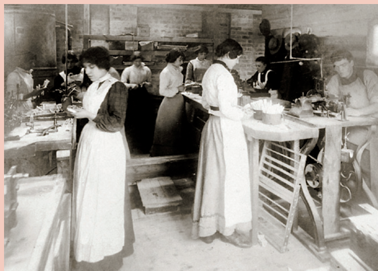
'A drilling shop. Boring tooth brush handles.' W. R. Tilbury & Co, Brush Manufacturers, Hackney, London, England. With thanks to BDA Museum.
