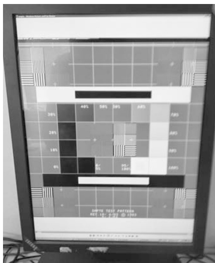
Fig. 2 A Totoku monitor was one of the medical grade monitors assessed. (An advantage of medical grade monitors is that the screen can swivel to present images in portrait or landscape mode, in this photograph the test pattern has been displayed in portrait mode)
