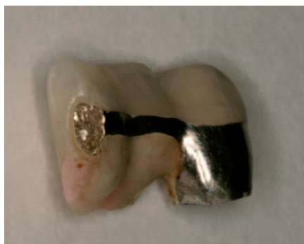
Fig. 14 Midline fracture of implant retained bridge replacing LR3-LL3. Metalwork is too thin in cross-section
