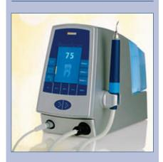
Sirona's PerioScan scaling system detects and gently removes subgingival deposits, minimising the risk of over-cautious/over-aggressive therapy. A new, all-in-one ultrasonic system for the detection and removal of dental calculus, the product detects deposits in places which dentists normally cannot view clearly – eg in the gum pockets.
