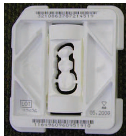
Fig. 3 Milled zirconia block
