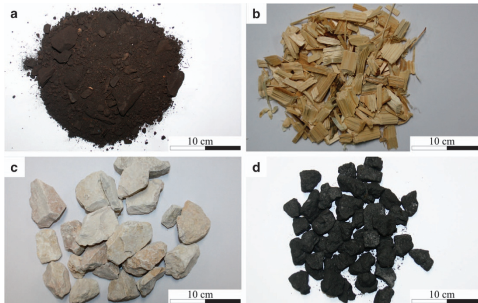
Figure 2. Sample photographs of the bulk solids I. (a) lignite, (b) wood chips, (c) limestone, (d) blast furnace coke (Figure from ref. 26).
